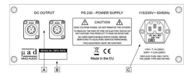
A. 6-PIN DC POWER SUPPLY OUTPUTS – This output allows interconnection of the LCPQ 4040 – MK2 unit. Up to two EQs can be connected to the power supply.
