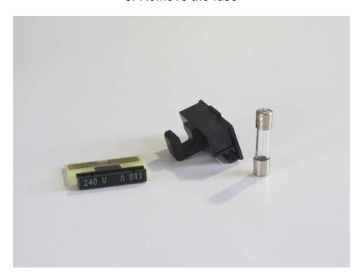
4. Insert the new fuse Always make sure you use the correct fuse type and rating!
