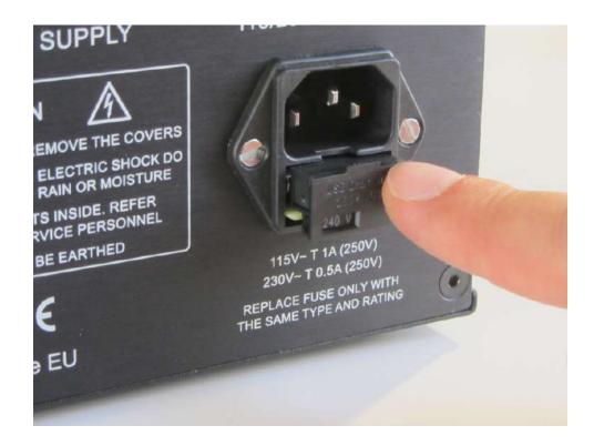
7. Make sure the fuse drawer is fully inserted into the power inlet.
