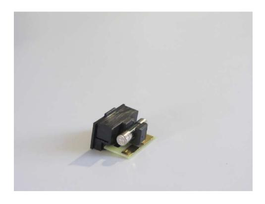
6. Insert the fuse drawer back into the Power Inlet
